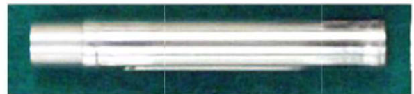
Fig. 1. Schematic drawing of an internal creep rupture specimen.
